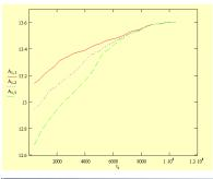
BLMG loading curves for 3 different charged batteries. BLMG takes care that all of the batteries reach homogenous voltage capacities after a short time.
